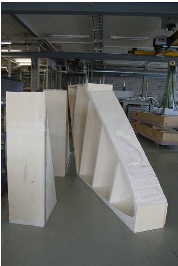
egg-shell prototypes PUR foam Blown with Solkane® 365/227 blend
