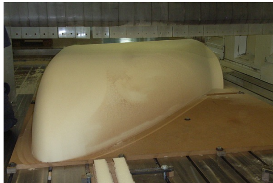
egg-shell prototypes PUR foam Blown with Solkane® 365/227 blend
